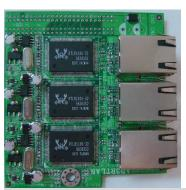
**AD3RTLAN-P/AD3RTLAN-G**For 2<sup>nd</sup>, 3<sup>th</sup>, 4<sup>th</sup> 10/100 or 10/100/1000 Ethernet LAN
